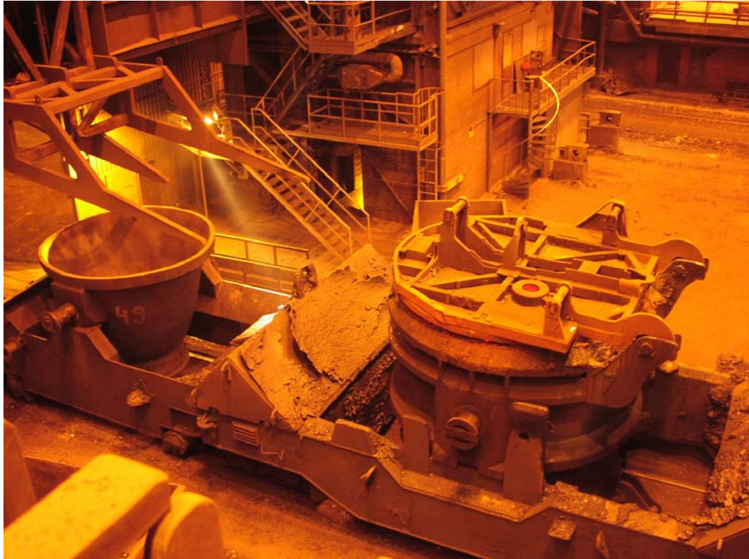
Figure 11. Automatic ladle lid system
