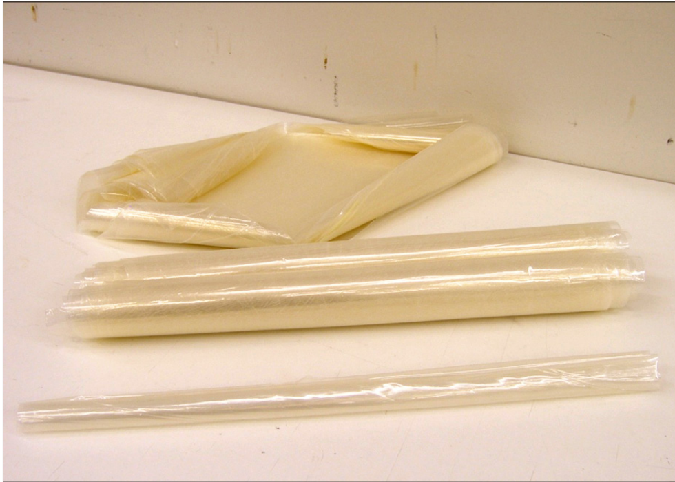
Figure 22. 20 g/m 2 PP coated dispersion coated plastic sheets. In front 3x glucose, back 1x glucose.
